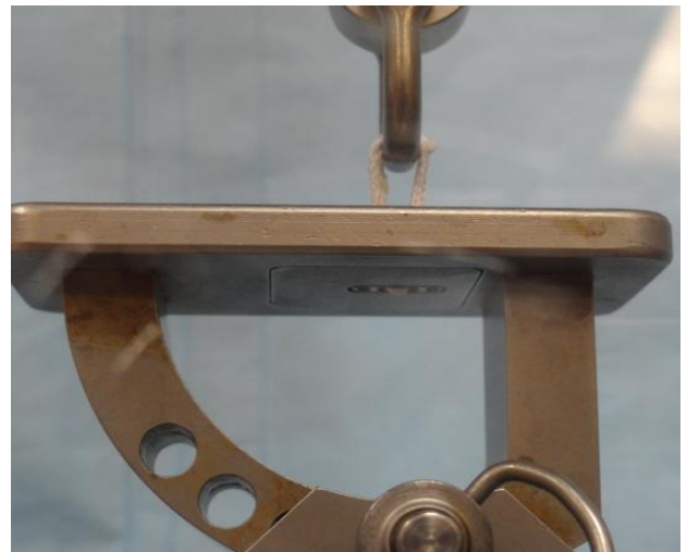
Figure 2: Close up view of test set-up showing shackle with loop and metal test plate.
